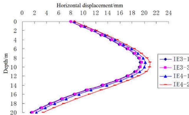
Fig.2 Variation curves of horizontal displacement of wall under 20 kPa overload in different periods
