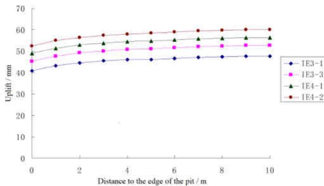
Fig.6 Variation curve of soil uplift in the pit with time under 50KPa load
