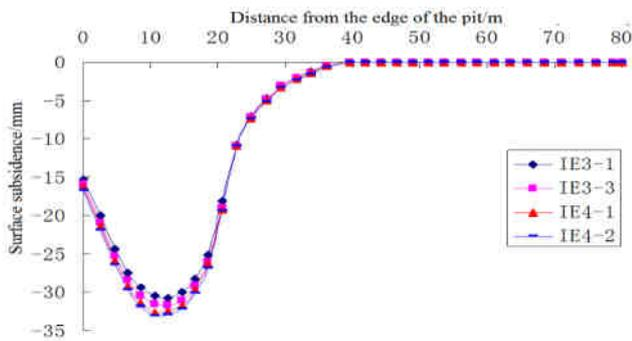
Fig.4 Variation curves of ground surface settlement behind wall under 20 kPa overload in different periods
