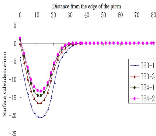
Fig.3 Variation curves of ground surface settlement behind wall without overload in different periods
