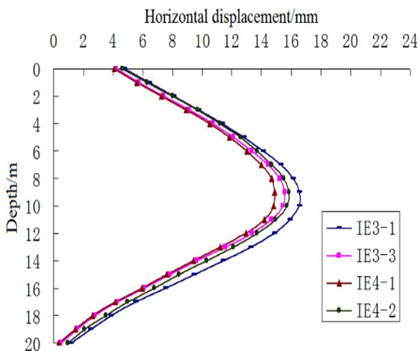
Fig.1 Variation curves of horizontal displacement of wall without overload in different periods
