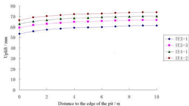
Fig.7 Variation curve of soil uplift in the pit with time under 70KPa load
