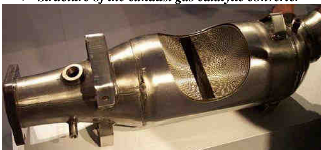
Figure 2.7. Structure of the exhaust gas catalytic converter [5]
