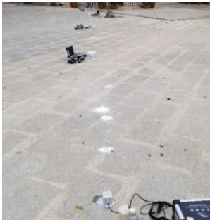
Fig.6 Partial measurement point of the vibration measuring instrument layout
