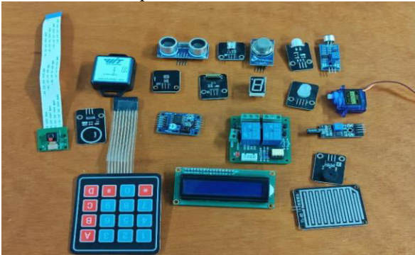
Fig. 8. Sensor modules used for junior secondary embedded-system inquiry activities.
