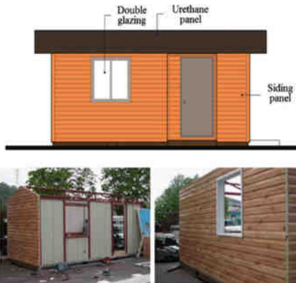
Fig. 4 Simple Design for Converting Shipping Container[4]
