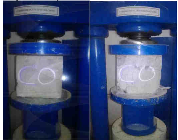
Fig1: : cube kept in CTM before testing (left) cube kept in CTM after testing (right)
