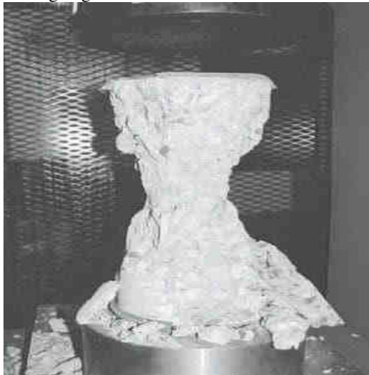
Fig.2: Fractured Concrete Cylinder Specimen at Failure
