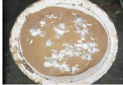
Figure 2: PP Fiber Mixed With Soil Sample
