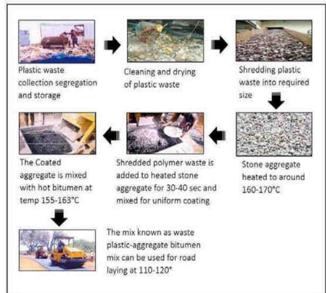
Figure 3: flowchart of plastic bitumen road process
