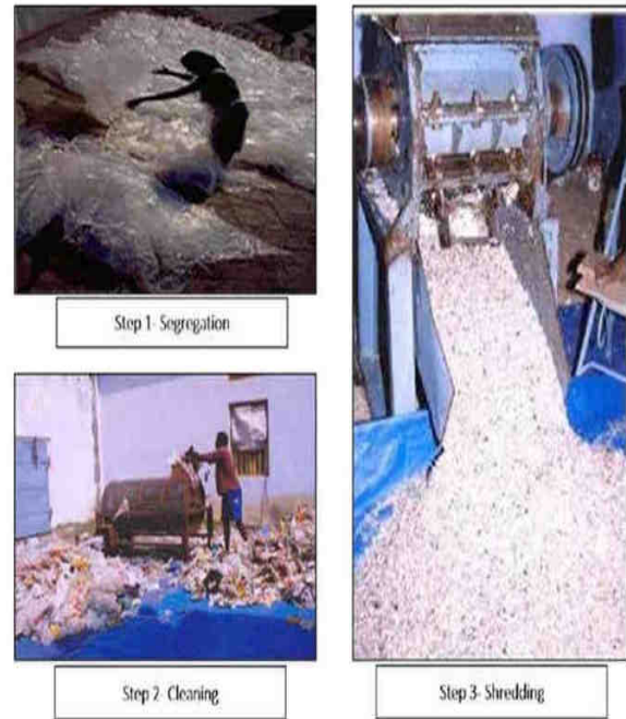
Figure: Steps to shred plastic waste for recycling purpose
