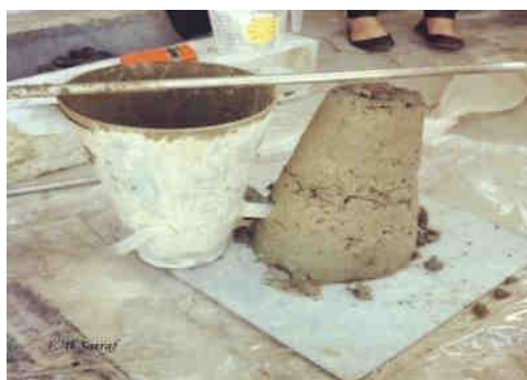
Fig. 2 Slump cone test
