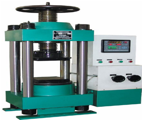
Compressive Testing Machine
