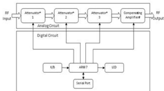
Fig.1 Block diagram of programmable digital attenuator.
