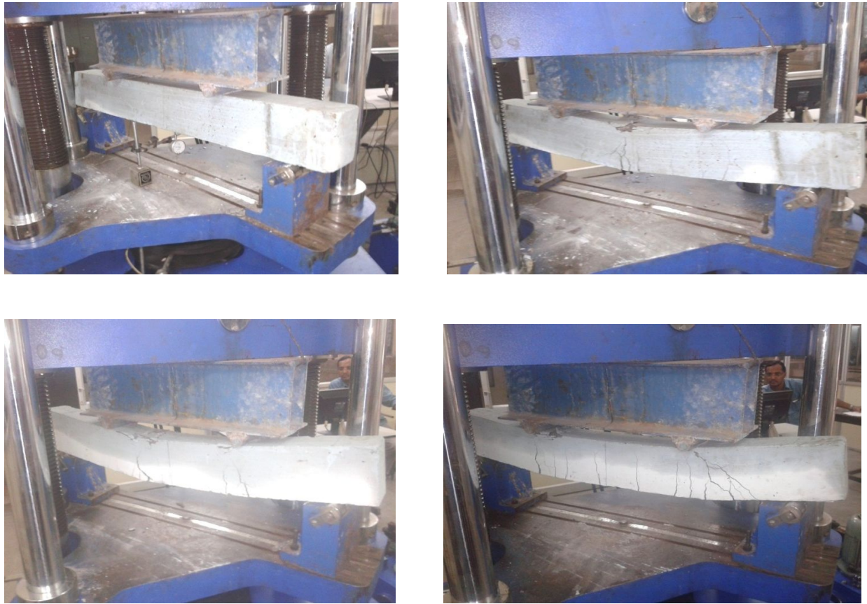
Figure 3: Flexural Test Setup
